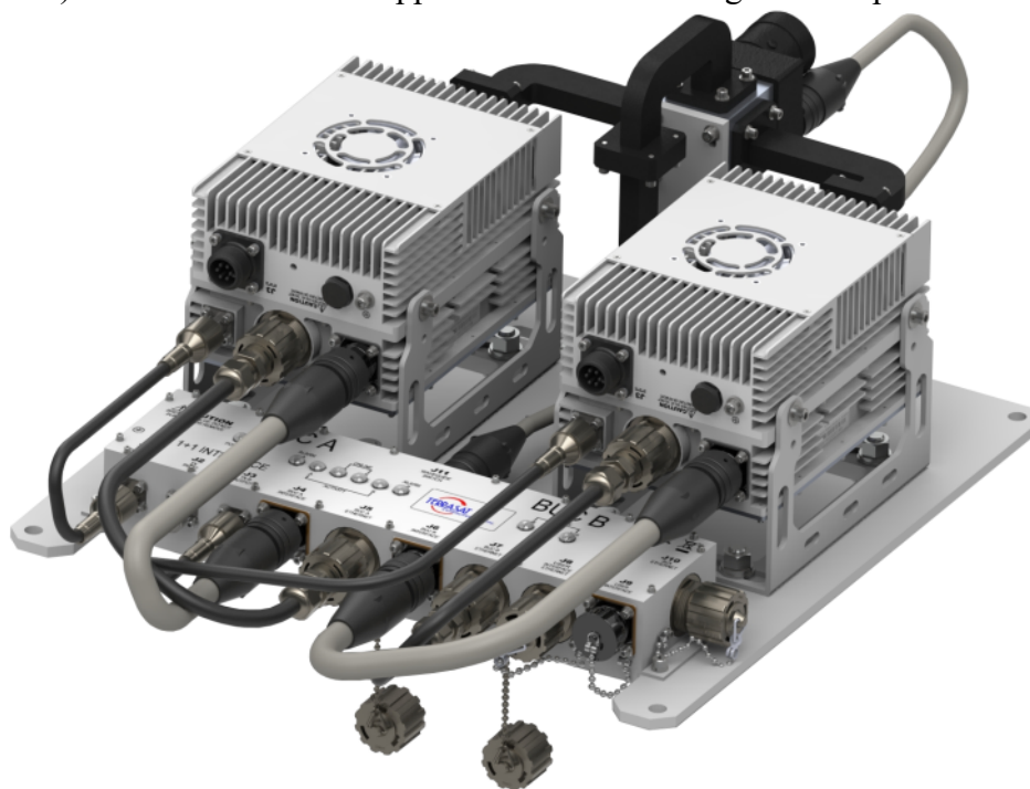
Figure 7.1 Transmit Redundant System Setup
