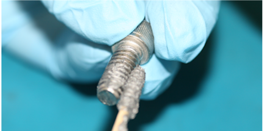
Figure 3.7 Applying the Anti-Seize Lubricant
